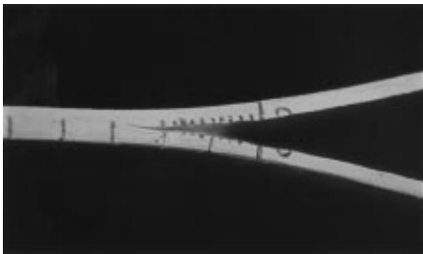
Figure 4 Fibre bridging during a Mode I test. The crack front is seen to be slightly bent out of plane and crack propagation followed the undulated paths of the warp yarns.
